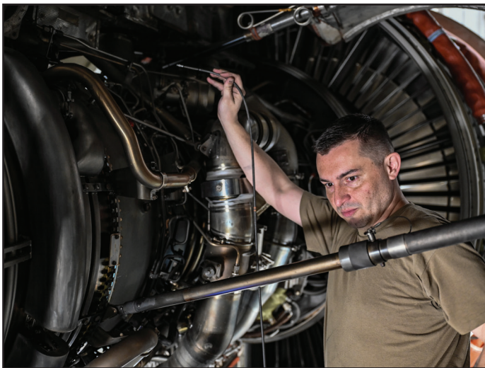
(left) Senior Airman Hunter Shaw, 445th Aircraft Maintenance Squadron aircraft hydraulic specialist, uses a torque wrench to tighten a nut on the front hydraulic strut of a C-17 Globemaster III at Wright-Patterson Air Force Base, March 16, 2025. A torque wrench is used to ensure fasteners like nuts and bolts are tighten to a specific, predetermined torque value, which is crucial for safety, proper assembly, and performance of equipment. They prevent both overtightening and under tightening.
