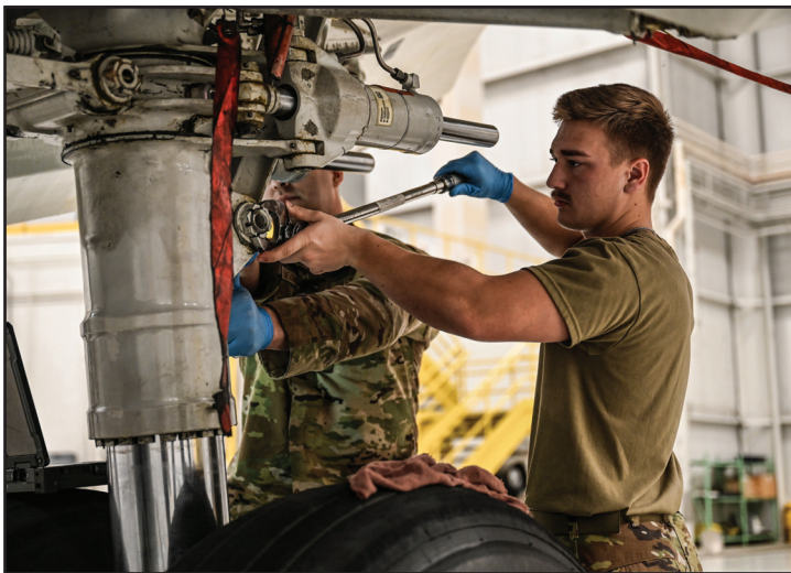
(left) Senior Airman Hunter Shaw, 445th Aircraft Maintenance Squadron aircraft hydraulic specialist, uses a torque wrench to tighten a nut on the front hydraulic strut of a C-17 Globemaster III at Wright-Patterson Air Force Base, March 16, 2025. A torque wrench is used to ensure fasteners like nuts and bolts are tighten to a specific, predetermined torque value, which is crucial for safety, proper assembly, and performance of equipment. They prevent both overtightening and under tightening.
