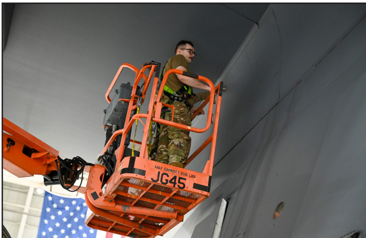
(left) Senior Airman Ethan Cass, 445th Aircraft Maintenance Squadron aerospace propulsion technician, stands on a lift while assisting a fellow Airman in riveting a panel on to the side of a C-17 Globemaster III at Wright-Patterson Air Force Base, March 16, 2025. A leaking fuel cell was replaced on the aircraft underneath the panel.
